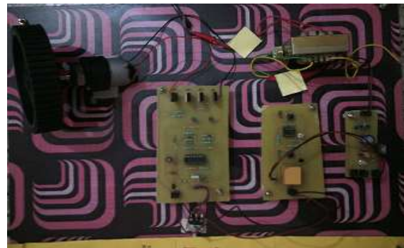
Fig 6:- Experimental setup of four quadrant operation
